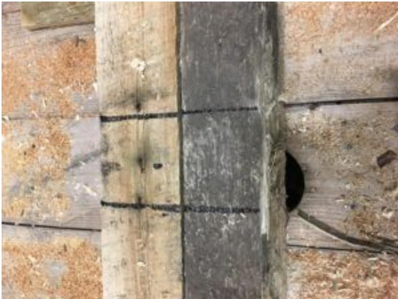
4. Once your pieces look like the pieces in the picture above, you can then begin to knock all of the excess wood out of the joint using a hammer, and then carefully with a knife or a chisel clear out all the remaining strips of wood at the bottom until the piece is clear and clean.
